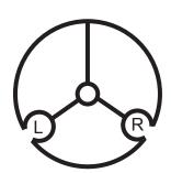
If a single section rack is to be mounted, half of all cornerpillars shall have the shelfbracket(s)mounted to the left (L) slot and the other half to the right (R) slot.
