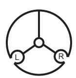
If a single section rack is to be mounted, half of all cornerpillars shall have the shelfbracket(s)mounted to the left (L) slot and the other half to the right (R) slot.
