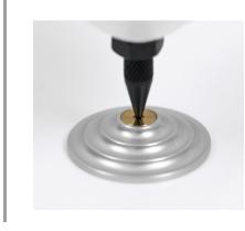
The smallest feet from Solid Tech is made out of anodized aluminum with a brass insert for the rack or loudspeaker spike. The brass insert will avoid any non-desired resonance from the floor to prolong into the rack and equipment. The design is pure and simple to suite all Solid Tech racks and loudspeaker stands.
