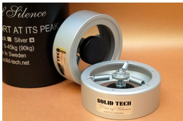
**BITS AND PARTS:** The pictures of the units pretty much tell you what you get for your money. Each of the cylindrical frame is nicely cut from aluminium, perforated to allow each of the ends of the springs to be mounted. The review units had three springs each, but these can be doubled for use with heavier equipment (alas, additional springs need to be purchased separately).
