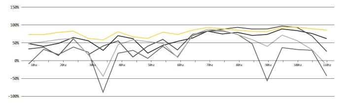
The graph above shows the average peak values of isolation efficiency stability across the frequency range of 10–115Hz, comparing the Feet of Balance with several alternative isolators.
