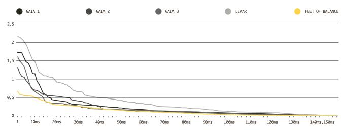
The graph above displays the damping decay time. The six different isolators are tested with a load within 10% of their maximum capacity. Each foot has been subjected to an impulse of 33g from a height of 1meter.
